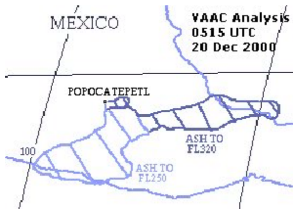
Figure 2. VAAC analysis near the time of MODIS image in Figure 1, based on animation of multi-spectral GOES imagery.
